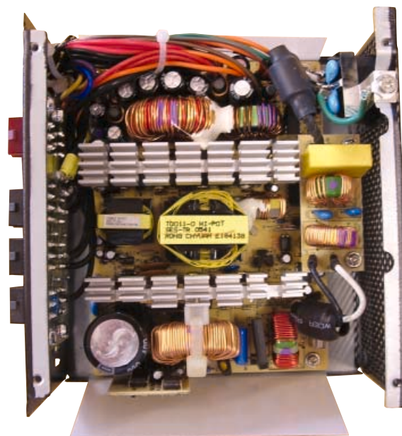
Power supplies may use fairly basic technology, but they're vital for your PC's reliability. This picture shows what a typical PSU looks like inside
